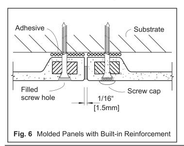
3) Provide a 1/16" [1.5mm] joint gap between panels - use spacers to maintain a consistent gap.
