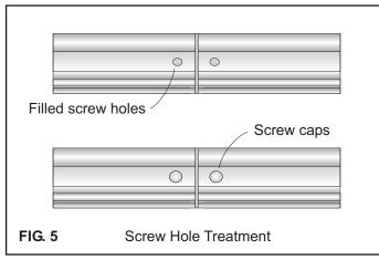
5) When a series of face fasteners are to be used, such as on panels or running trim, evenly space the screw holes apart for improved aesthetics.
