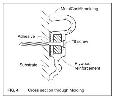
4) Screw holes can be filled with MetalCast® 2-part patching compound. Follow hole patching instructions. Note: Screw holes filled with MetalCast® patching compound will remain visible afterward. Alternatively,
